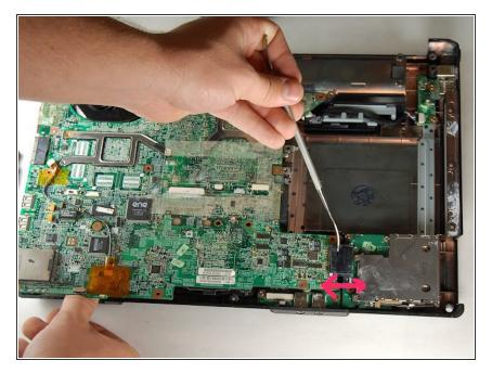
• Separate the motherboard from the rest of the components.
