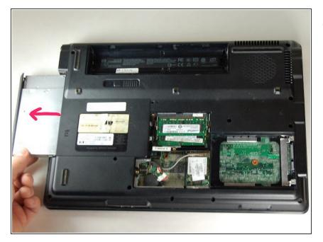
After removing the back of the memory card and the back of the hard drive, remove the CD Drive by gently pulling it all the way out of the device.
