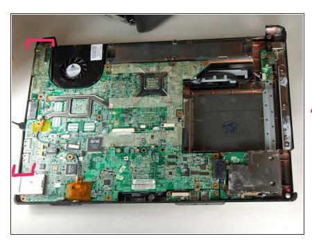
After all screws are removed use metal spudger to pry the plastic housing away from the ports to separate.
