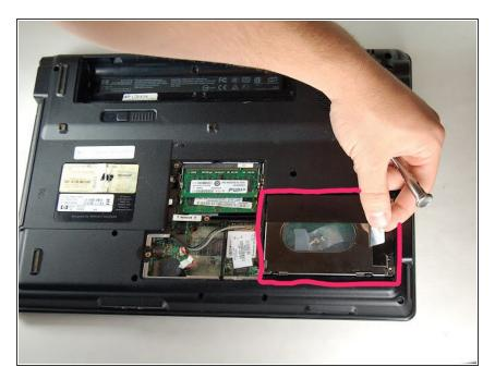
After removing the backs of the memory card and hard drive cover, gently remove the silver screen.
