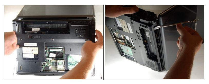
• After all components are removed, use your hands to separate the base plate form the main housing. If your fingers can not separate the 2 pieces; insert the metal spudger to create space.
