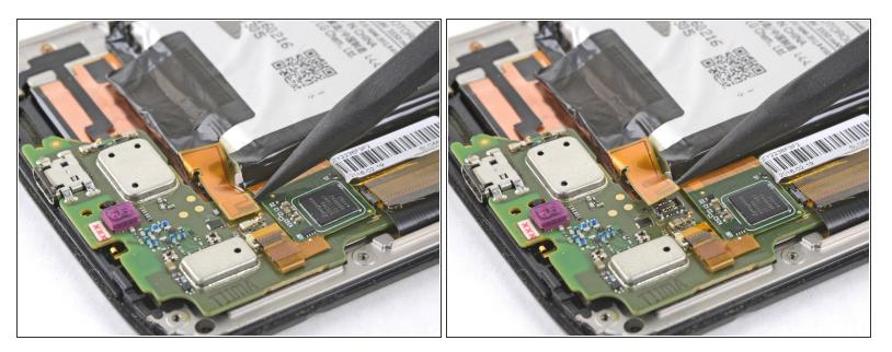
• Use the point of a spudger to pry up and disconnect the battery pack connector.
