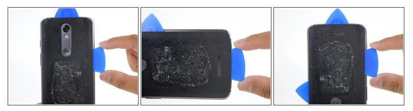
Repeat the iOpener heating and slicing procedures for the remaining three sides.
