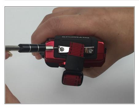
Locate the strap eyelet side of the camera and use the PH000 screwdriver to remove the two
