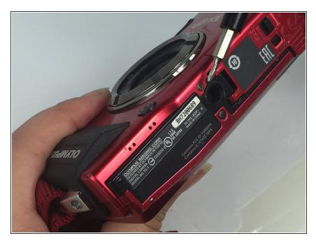
Locate the bottom section of the camera. Using the PH000 screwdriver, remove the two 4mm screws located towards the middle (near the battery compartment).
