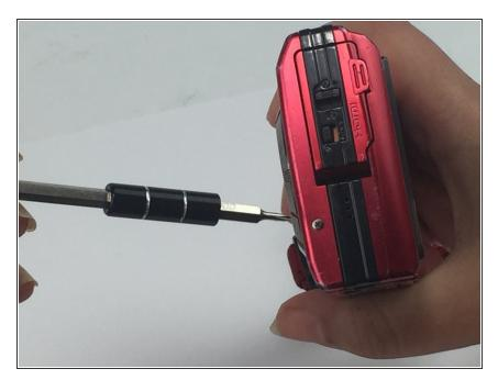
Locate the side of the camera containing the HDMI port. Use the PH000 screwdriver to remove the 5.4mm screw located on the lower left side below the port.
