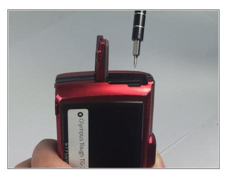
Using the PH000 screwdriver, remove the 3.8mm screw located inside the HDMI port.
