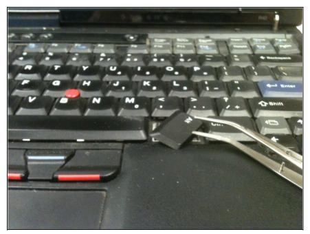
• Locate the key that needs replacing. Use tweezers to slowly pull the key off the keyboard. Doing this will expose the underside of the keyboard.
