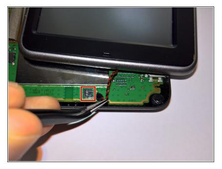
Lift the connector gently from the socket, making sure you pull in the right direction.
