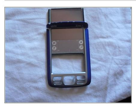
Remove the screen from the front housing and set it aside.
