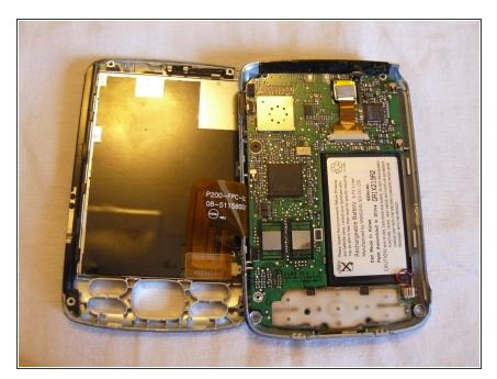
Pull the back panel off the body of the unit to expose the motherboard in the body.
