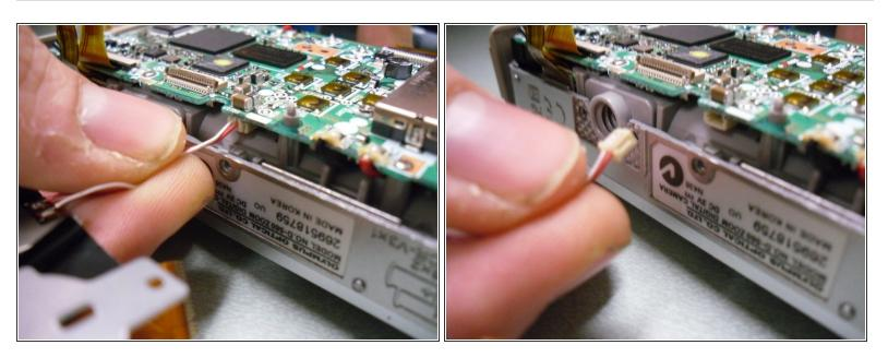
Unclip the plug attached to the red and white wires that connects the LCD screen to the motherboard.
