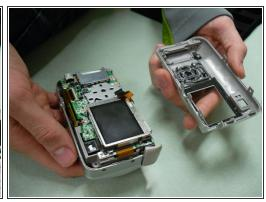
Use the plastic opening tool to separate the back cover from the camera.
