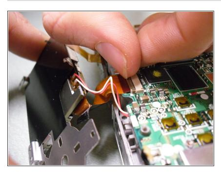
Undo the clip holding the ribbon cable that attaches the LCD screen to the motherboard.
