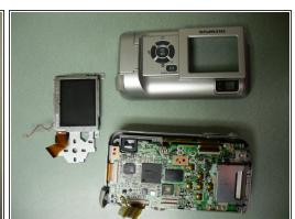
• The LCD screen housing should now be free of the camera.
