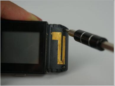
Use a PH000 screw head to undo the newly revealed 4 mm Phillips screws that were hidden beneath the glue. To reassemble your device, follow these instructions in reverse order. Keep in mind that you will need to cut the band for this guide and it cannot be reattached.
