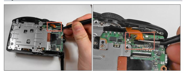
• Gently detach the flex ribbon with your tweezers before removing the front plate.
