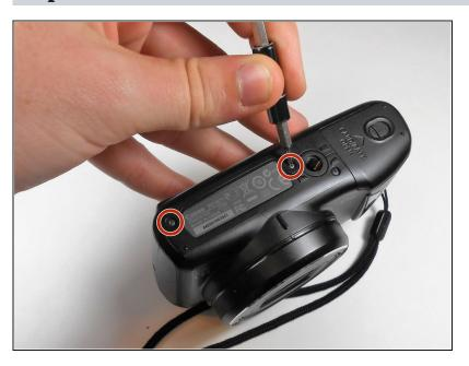
Remove two 4mm screws from the bottom of the camera with the J000 head screw driver.
