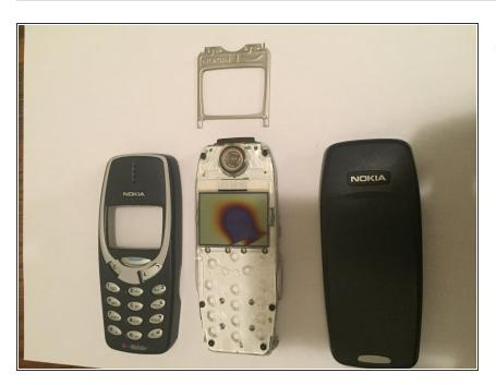
Remove the metal casing
