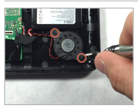
Unscrew the two 5mm screws using a Phillips #000 screwdriver.
