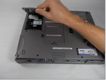
• Unscrew the one Phillips #0 screw at the bottom of the panel and remove the panel.
