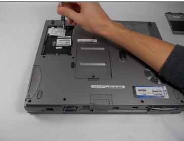
• Unscrew the two 3mm Phillips #0 screws located on the card.
