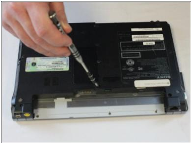
Remove one 5 mm Phillips #1 pan head screw, in the middle of the laptop, using a Bit Driver with Phillips PH1 bit.
