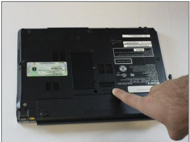
• Slide battery release toggle switch towards the "RELEASE" print.
