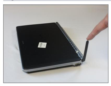
Swivel the Network Antenna up so that it points upward.
