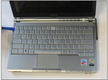
$\triangle$  Be sure to pry the plastic opening tool under the keyboard, rather than under the keys. Otherwise, some keys could get harmed.
