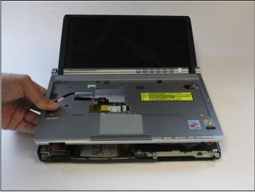
Disconnect the ribbon cable by pulling straight up with your fingers.
