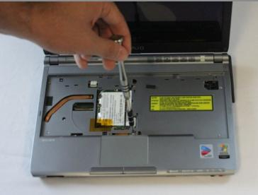
• Remove one 7 mm Phillips #1 Pan Head Screw by using a Bit Driver with Phillips PH1 bit.
