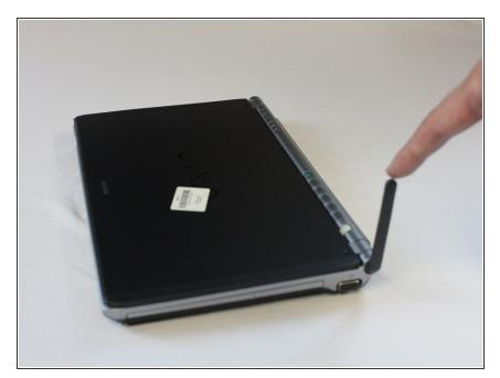
Swivel the Network Antenna up so that it points upward.
