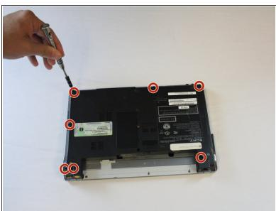
Remove seven 5 mm Phillips #1 pan head screws with a Bit Driver, using a Phillips PH1 bit.
