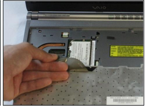
**⚠ Do not pull the keyboard too far away, as a ribbon cable is still attached. Failing to do so can cause damage to the ribbon cable or the connector.**
