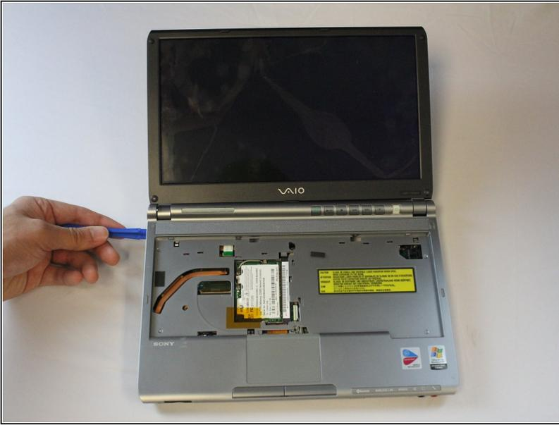
⚠ Do not pull the plastic cover too far away, as a ribbon cable is still attached. Failing to do so can cause damage to ribbon cable or the connector.
