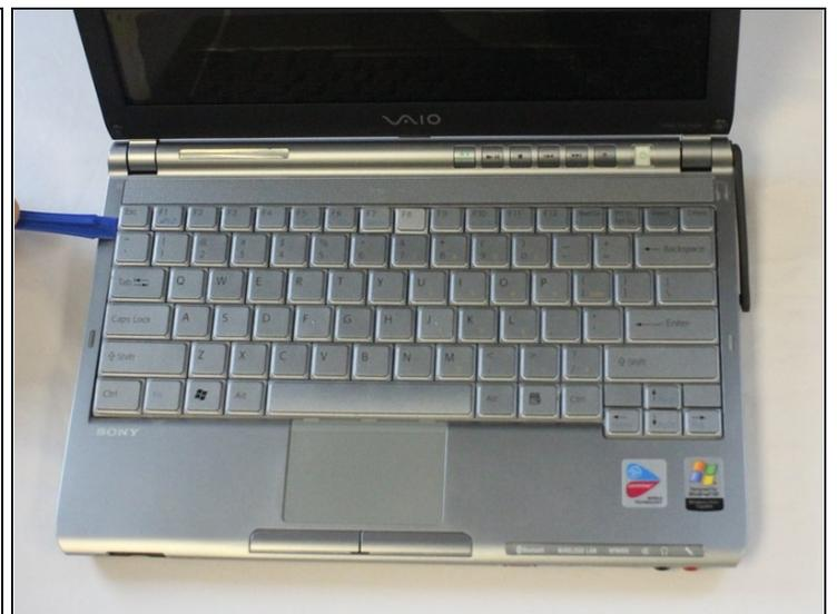
⚠ Be sure to pry the plastic opening tool under the keyboard, rather than under the keys. Otherwise, some keys could get harmed.
