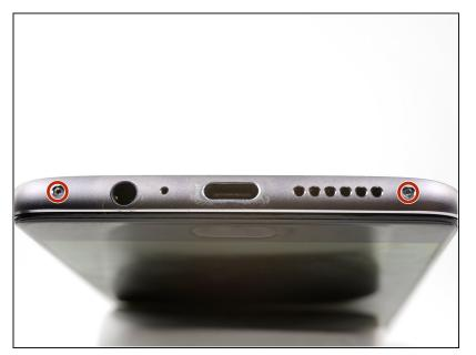
Remove the two 2.6 mm T2 screws from the bottom edge of the phone.
