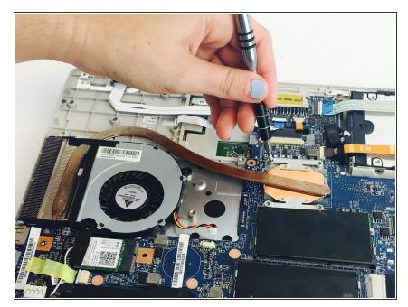
• Unscrew the two 3.75mm screws around the Cooling Fan and the copper attachment as shown with the #0 Phillip's Head screwdriver.
