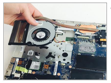
Remove the attachment from the Processor by gently rotating and lifting.
