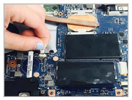
Disconnect the Cooling Fan from the Motherboard by gently pulling away on the white tab.
