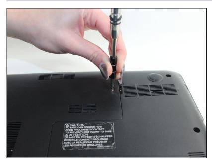
Using a small Phillip's head screwdriver, unscrew the single 7 mm screw (5 mm head) on the L-shaped panel on the backside of the laptop.
