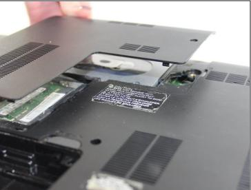
• Once the screw is removed, pry the panel upwards by gripping the groove pictured.
