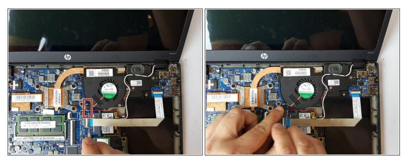
Remove the connection from the fan to the motherboard by using the nylon spudger or your fingers.
