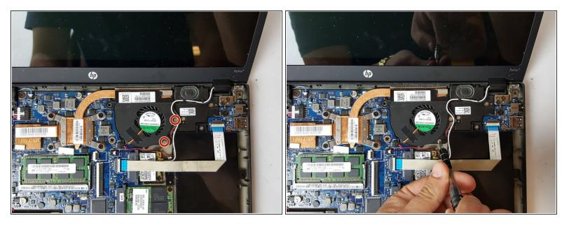
Use a PH1 screw head to remove the two, 3mm screws.
