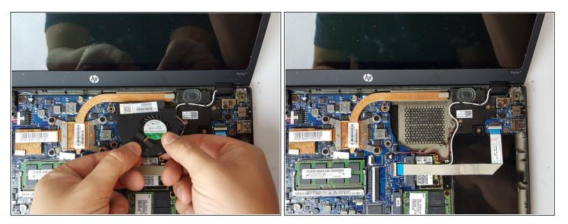
• Remove and replace the cooling fan.
