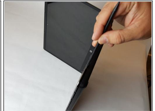
**i** This step requires unlocking the very fragile plastic clips along the frame; take care not to damage them.
