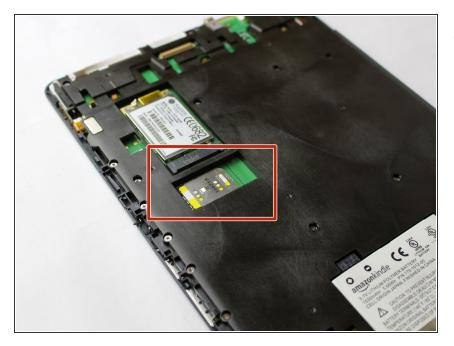
• Locate and remove the SIM card slot.
