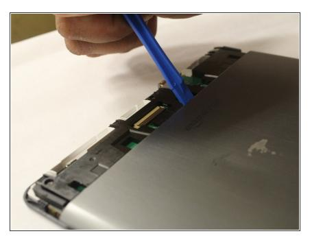
• Use the plastic opening tool to take the off the metal plate.
