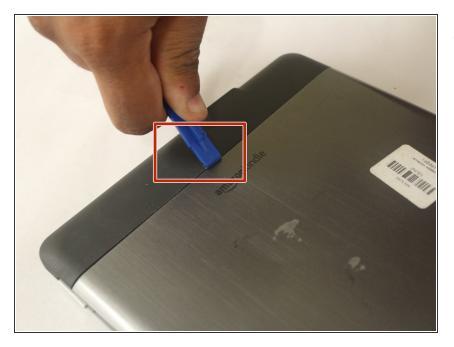
Use the plastic opening tool to push against the top part of the e-reader to open the device.
