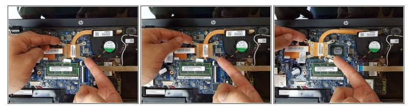
• Remove the heatsink with you fingers and replace it with a new heatsink.
