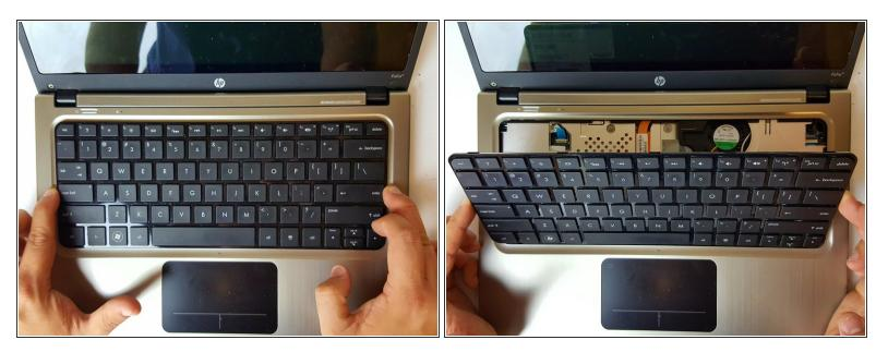
Slide the keyboard up and towards the screen just enough to separate the keyboard from the top cover.
