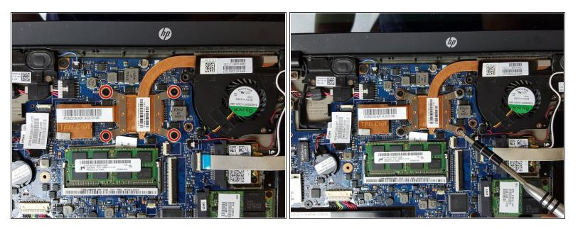
Use a PH1 screw head to take out the four, 2mm screws.
