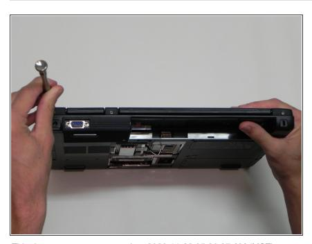
Lift the laptop to be on its edge, with the bottom of the screen in the air.
