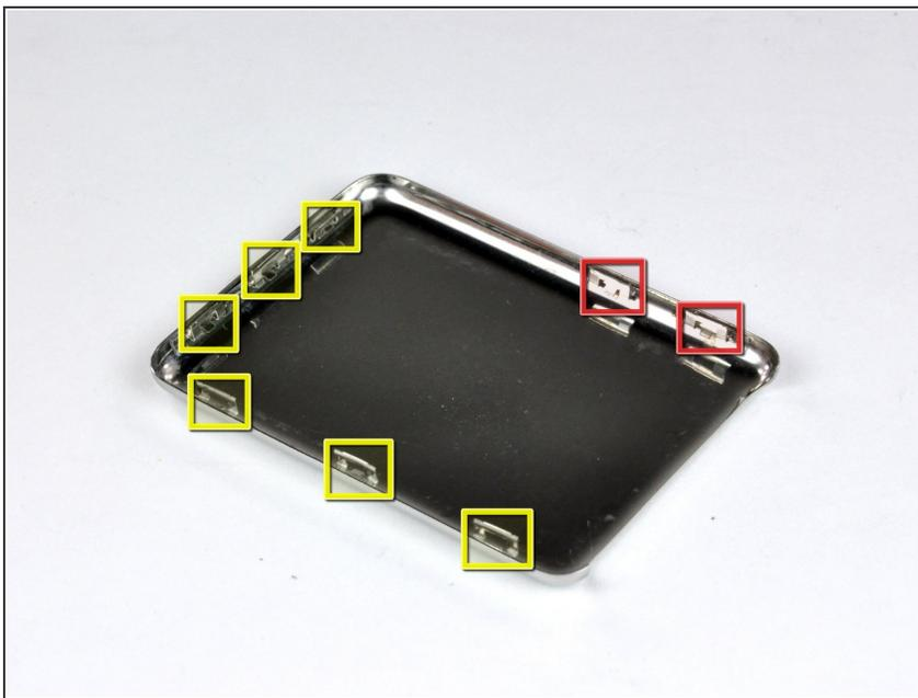
**i** The rear panel is secured to the front case by eight clips permanently attached to the rear
