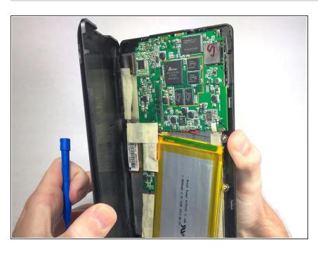
Pull the cover off of the device once about three quarters of the cover has been pried open using the plastic opening tool.
