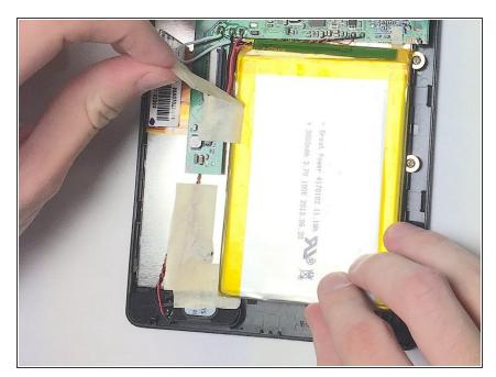
Remove masking tape from the battery.
