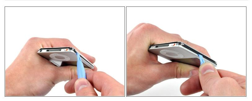
(i) The large iPod opening tool is no longer needed to gain access to the left side of the iPod.
