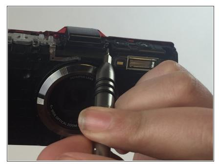
Use the PH0000 screwdriver to remove the 7 mm located on the upper side of the camera, where the shutter and zoom bottoms are. You will find the screw towards the middle of this section.
