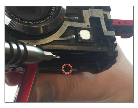
Use a PH000 screwdriver to remove the 3 mm screw located on the bottom of the battery compartment.
