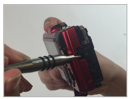
Using the PH000 screwdriver, remove the two 4mm screws located on the left side of the camera, under the strap holder.
