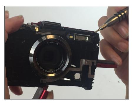
Use a PH000 screwdriver to remove the 6mm screw on the upper right side of the camera, above the flash.
