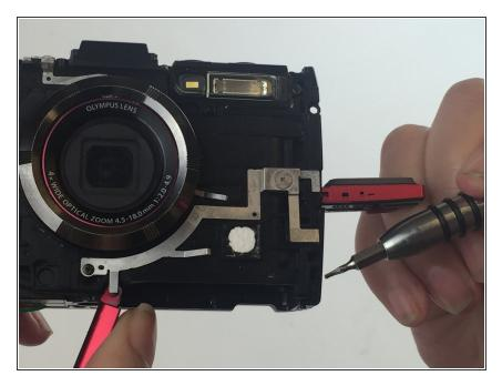
Using the PH000 screwdriver, remove the 1.2 mm located on the lower right side of the device, towards the corner.
