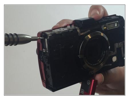
Hold the device as shown in the picture. Using the PH000 screwdriver, remove the 9mm screw located on the upper left side of the camera.
