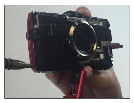
Use the PH000 screwdriver to remove the 7mm screw you'll find toward the lower left side of the camera.
