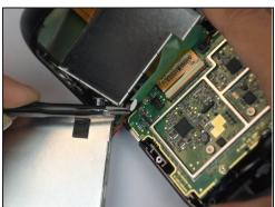
Remove the battery connection.
