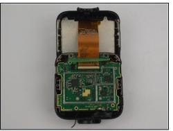
• Remove the three 5 mm screws using the Torx T5 screwdriver.
