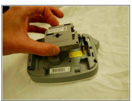
■ To remove the label cartridge from the device, use a plastic opening tool from your iFixit tool kit.
