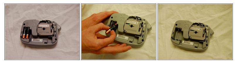
• Remove the batteries from your device.
