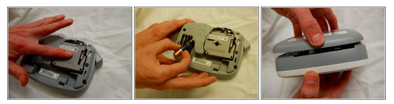
Place the label cartridge and batteries back into your device. Refasten the bottom case of the label-maker.
