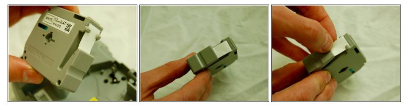
• Press the label paper back into alignment with the small holders on the right side of the label cartridge.
