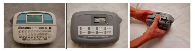
• Turn your label-maker on its face. Using your thumb, press in and then upward on the fastener located on the side of your device.
