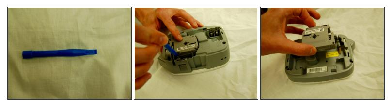
• Using a plastic opening tool from your iFixit tool kit, leverage the label cartridge out of your device.
