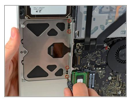
While holding the edge of the trackpad closest to the logic board with one hand, remove the four 1.2 mm Phillips screws highlighted in red.
