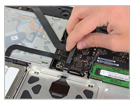
Use the flat end of a spudger to carefully pry the trackpad connector up from its socket on the logic board.
