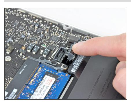
Bend the battery cable slightly away from its socket on the logic board so it does not accidentally connect itself while you work.
