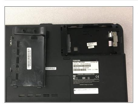
Once the cover is off, the hard drive will be exposed, carefully pull it out to the right.
