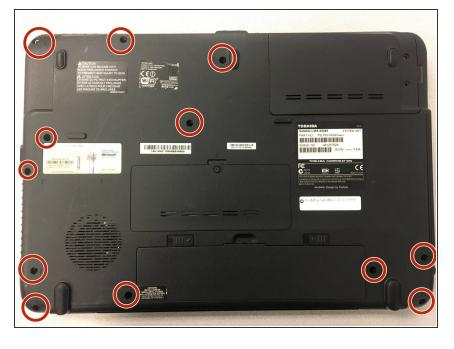
Start on the back and unscrew the 12 Phillips #0 11-mm screws holding the back cover down.
