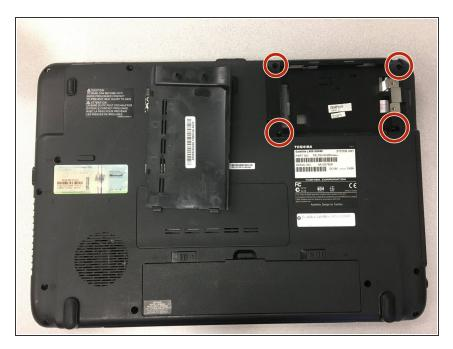
Pop off the hard drive cover, and then unscrew the four 11-mm
