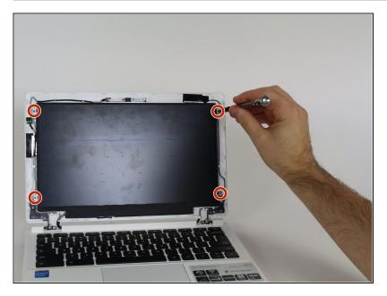
Locate and remove the four 4.2mm screws holding the screen in place by using a Phillips #1 screwdriver.
