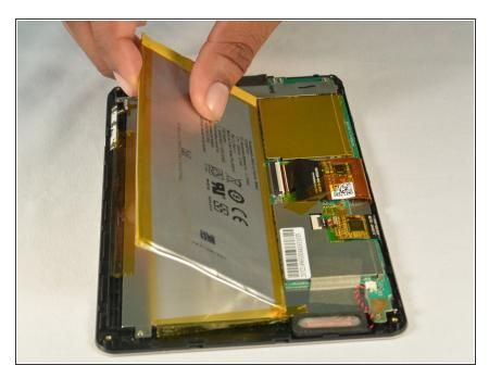
• Lift the battery from the device.
