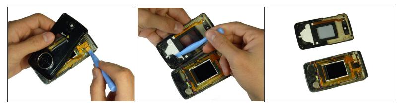
**Caution:** The wires and ribbon connector can break easily. Exhibit care when removing them.
