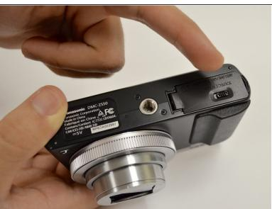
Turn the camera off and identify the battery door located on the bottom of the camera.
