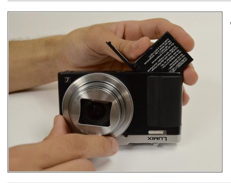
The battery should now be released; you may now remove the battery from the camera body.
