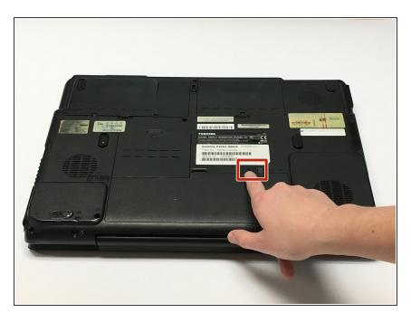
Slide the battery lock (marked with a 1), located at the top of the battery compartment, to the right.
