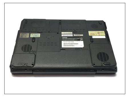
Place the laptop upside down on a flat surface with the screen closed.
