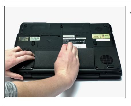
Lift the battery to completely remove it from the laptop.
