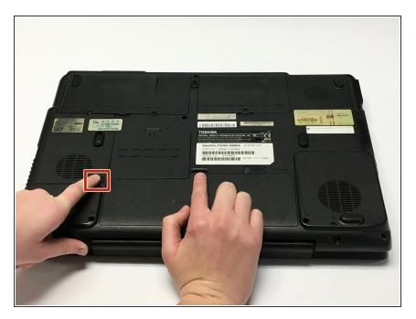
Slide the far left latch (marked with a 2) to the left and hold while lifting the battery upward.
