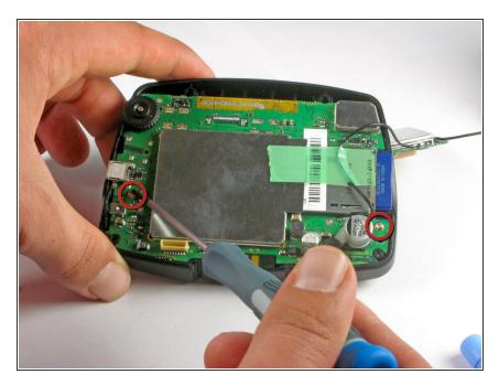
Remove the two Phillips #00 screws securing the motherboard to the front case assembly.
