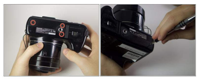
• Turn the camera upside down and unscrew the three 5mm screws found on the bottom.
