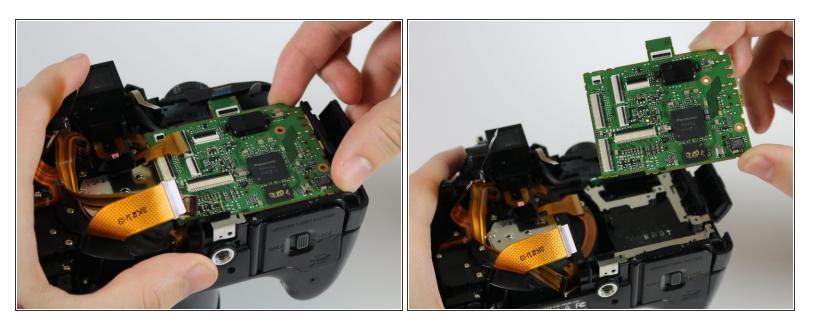
• Once the screws and the ribbon cables have been removed, lift the mother board from its slot.
