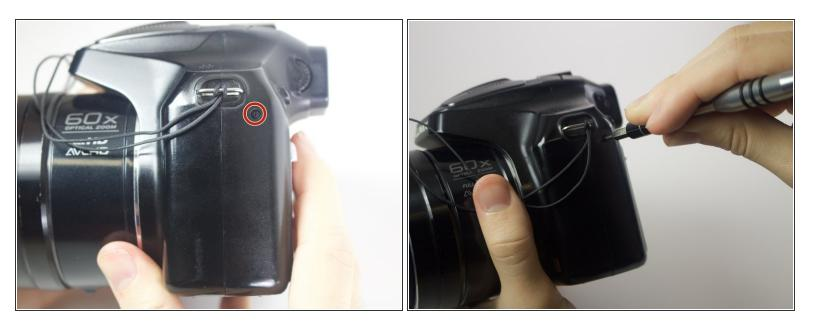
• Flip the camera over to the left side of the screen and unscrew the 5mm Phillips screw found there.
