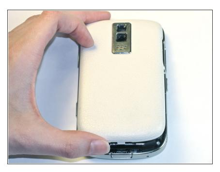
• Press the cover release button on the bottom of your device. Lift and remove the back cover.
