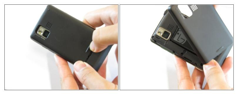
• Remove the back cover by firmly pressing against the raised lip on the back panel. Slide the cover towards the top of the phone.
