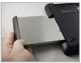
Unscrew one 3.85mm screw using the PH0 tip and remove from the disk drive.
