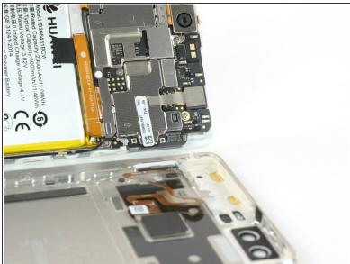
Disconnect the fingerprint sensor using a spudger.
