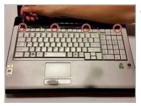
Use a PH0 screwdriver to unscrew the 4 screws at the top of the keyboard.
