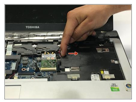
• Flip the computer back over and push the metal tab to the right to release the CD drive from its docking port.
