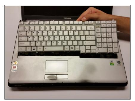
• Once the ribbon is released the keyboard can be removed .
