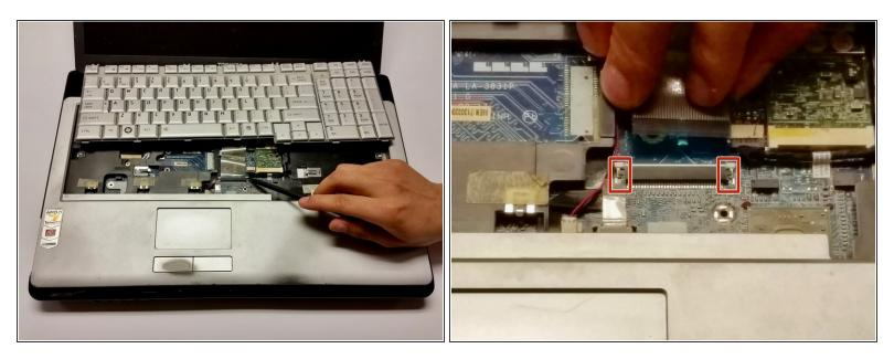
• To remove the ribbon cable, push upward on the small tabs located on either side of the ribbon.
