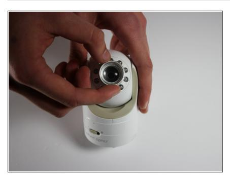
Place the replacement lens on top of the opening and twist to the right until it is secured.
