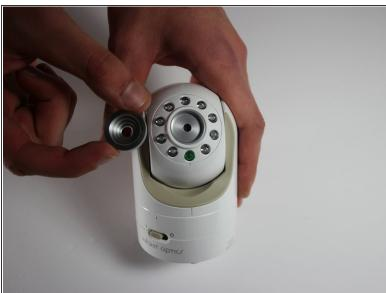
Grasp the lens with your index finger and thumb and twist to the left until it detaches.
