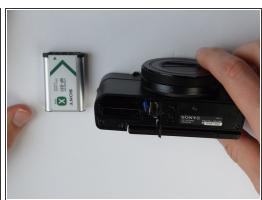
Remove battery by sliding the tab to open the cover
