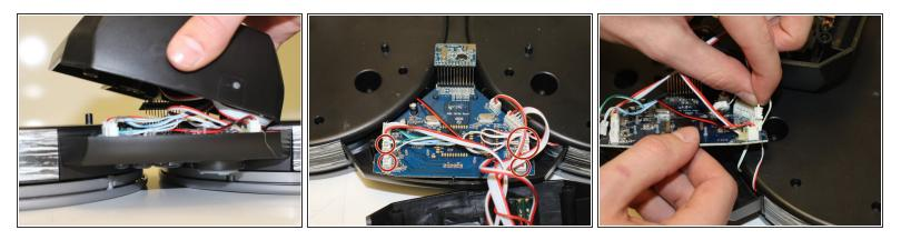
• Open the bottom module. Disconnect the five wire clips as shown in the pictures.
