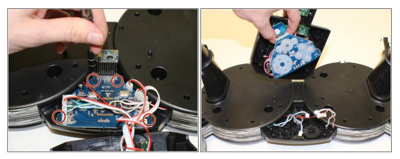
Remove the four Phillips #1 sized screws holding the main circuit board. Rotate the board up and out, exposing the buttons.
