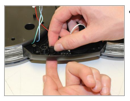
• The buttons can be pushed up from the bottom to be removed.
