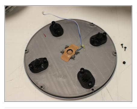
The sensor can be peeled off of the drum pad.
